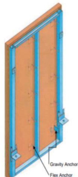
Typical stud frame fixing assembly
